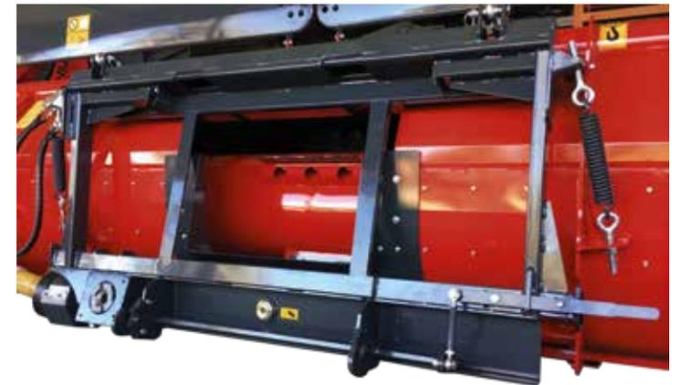
Leveling sensors and auger sensors are available on SPARTAN, depending on forage harvester capabilities and options.
