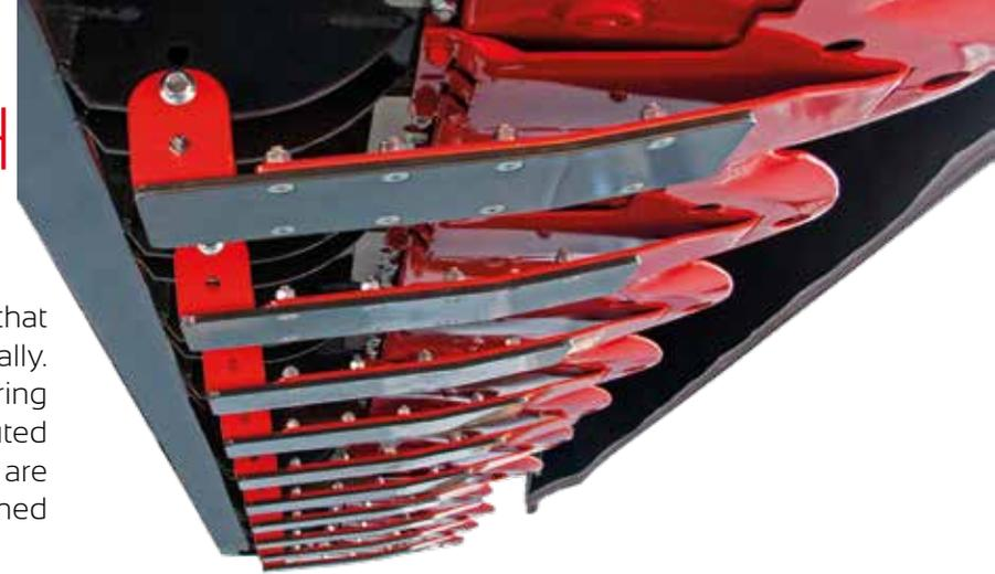
The fluctuating adapter plate enables the header to contour to the terrain. SPARTAN is adaptable to all kinds and models of forage harvester with a simple replacement of the adapter kit.
