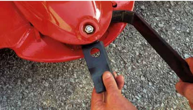
Quick-change knives dramatically reduce replacement time without the use of tools. Cutting discs are made to have a remarkably close proximity of knives and provide a perfect cut even with packed and wet product.
