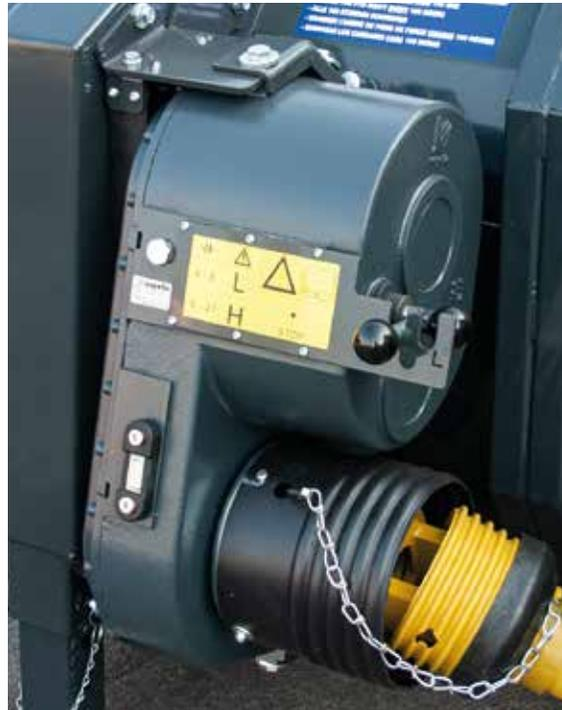
Continuous feeding: thanks to the integrated gearbox on all headers, it is possible to change the auger speed and cutting length of the harvest at the same time with a simple gear shift.
